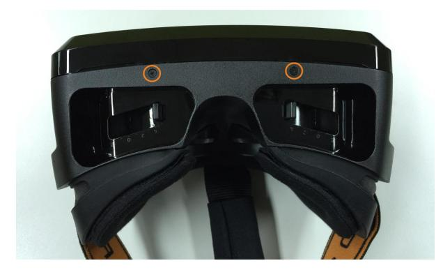
4. Remove the screws from the bottom of the HMD module.
