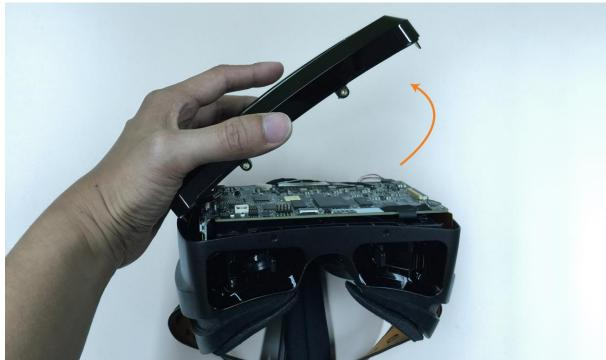
Note: It may require a bit of force to detach the magnetic locks. Avoid yanking the front panel so as not to damage the ribbon cable.
