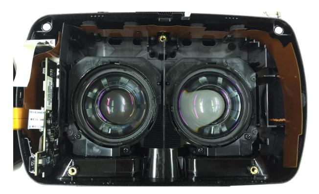
14. Flip and place the display module on your work surface.
