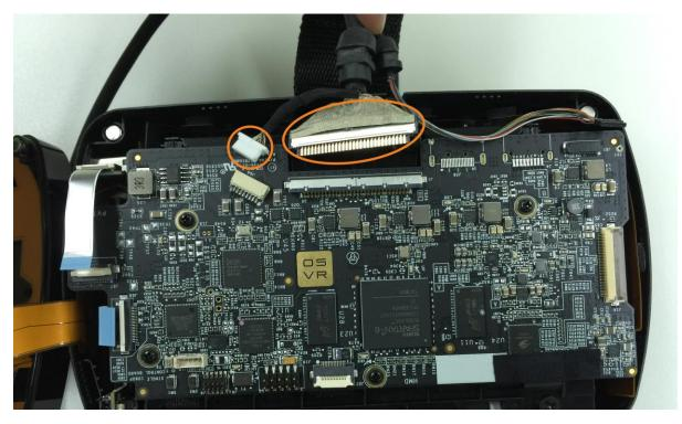
24. Gently place the rubber cables to the top of the HMD module.
