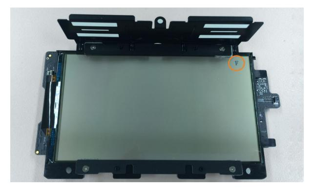
17. Peel a small portion of the back plastic cover of the film and place it on the display module.
