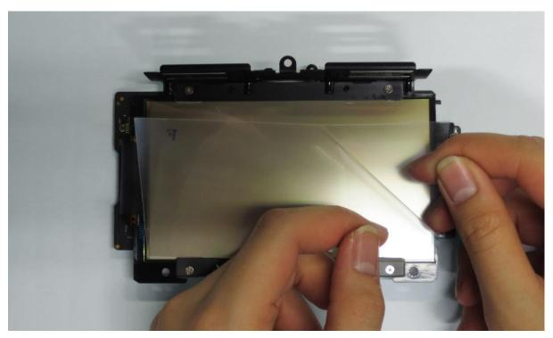
18. Starting from the middle, use the wiper to carefully push away the air bubbles trapped between the film and the display module.
