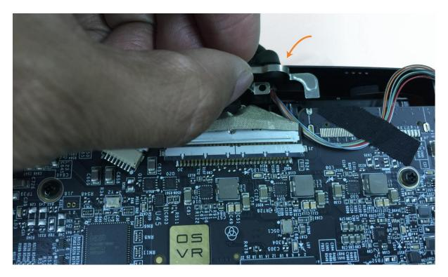
27. Carefully close the front panel of the HMD module.
