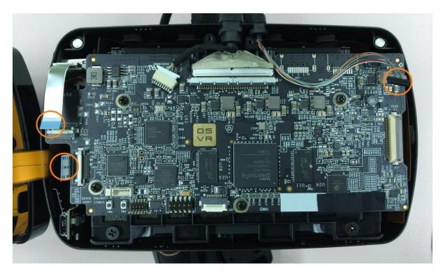
9. Gently lift the rubber cables from the top of the HMD module.
