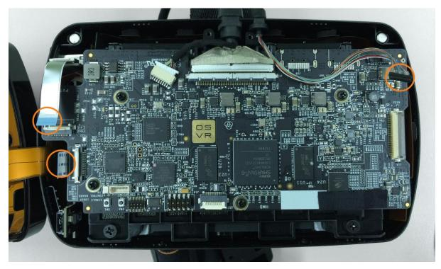
26. Place the cable holder to the HMD module.
