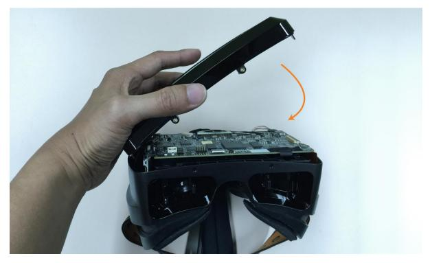
28. Reinsert the screws to the HMD module.
