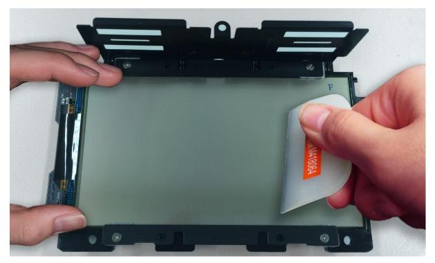
20. Carefully remove the front plastic cover to avoid peeling off the entire film.
