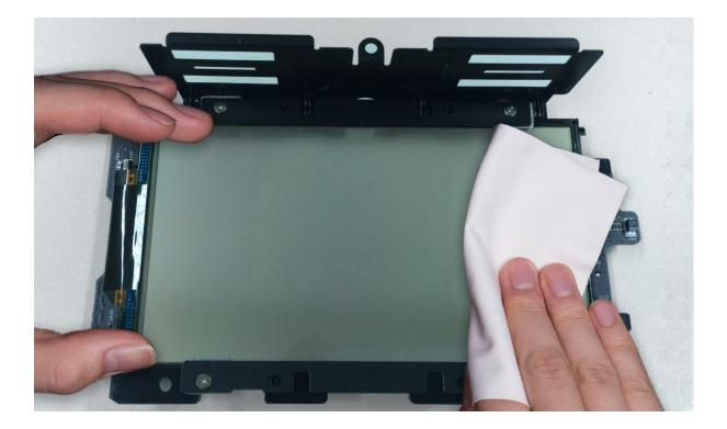
16. Without peeling, place the film with the "F" facing you on the display module to gauge the correct placement.
