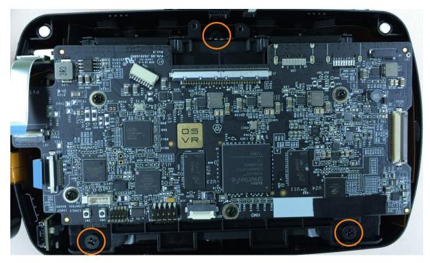
12. Carefully lift the display module.
