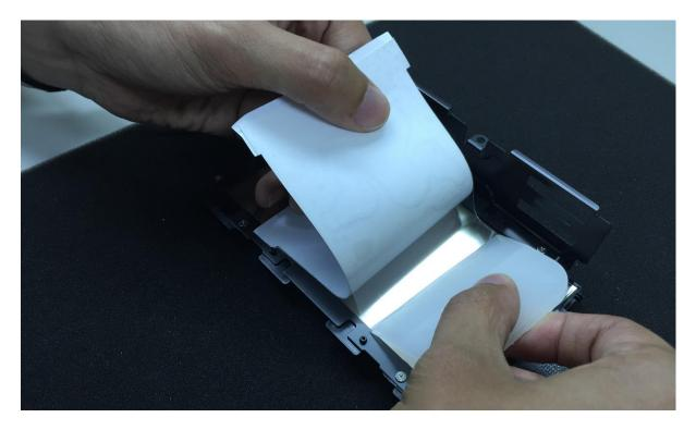
19. Continue peeling and removing the air bubbles until the film is fully applied to the display module.
