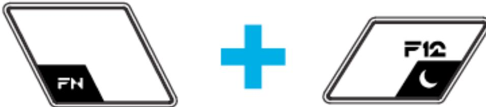
You can enter the Sleep mode quickly with your TRON Gaming Keyboard. Simply press “FN” button with the Sleep Mode button. To wake up from Sleep mode, press any key on your TRON Gaming Keyboard.
