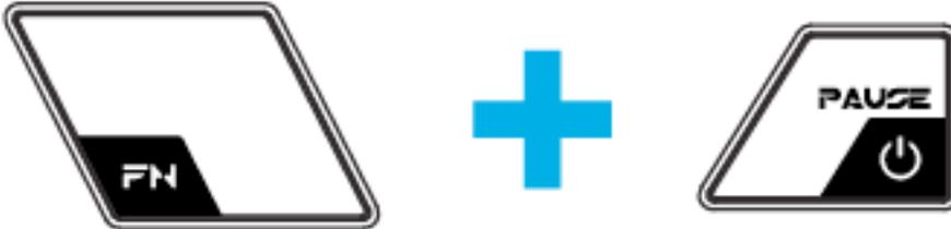
You can switch off your PC by holding the FN button and pressing the power button.
