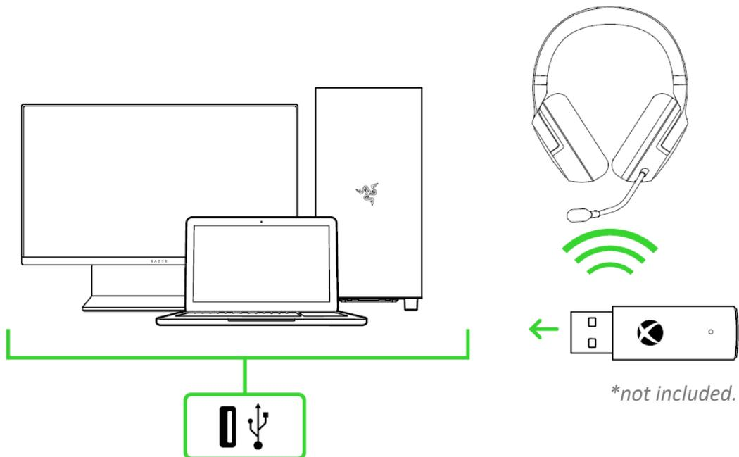
2. While powered off, press and hold the power button until the status indicator is lit, or until you hear a tone.
