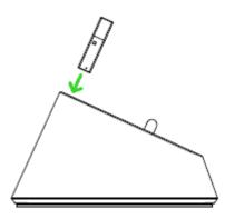
You can use the charging dock to replenish your mouse's battery and to extend the reach of your USB wireless dongle. You can also connect to Razer Synapse and place your Razer mouse on the charging dock to view the mouse's current battery status.
