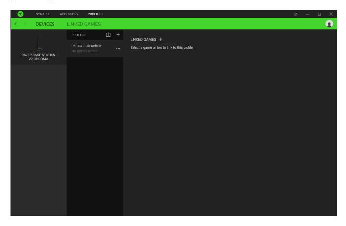
You can import Profiles from your computer or from the cloud through the import button ( ) or create new profiles within the selected device using the add button ( + ). To rename, duplicate, export, or delete a profile, simply press the Miscellaneous button ( • • • ). Each profile can be set to automatically activate when you run an application using the Linked Games option.
