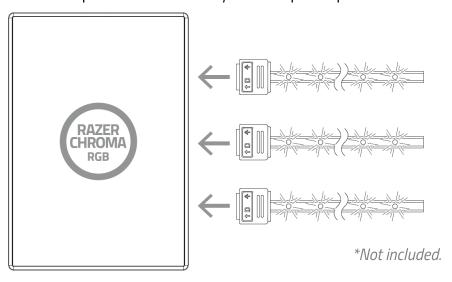
2. Connect the ARGB controller to the Molex socket of your PC's power supply unit using the Molex to DC cable.
