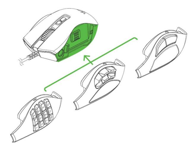
To customize each side plate's button assignments, please install Razer Synapse. These side plates are designed for the Razer Naga Pro only. Don't use side plates from the Razer Naga Trinity, and vice versa.
