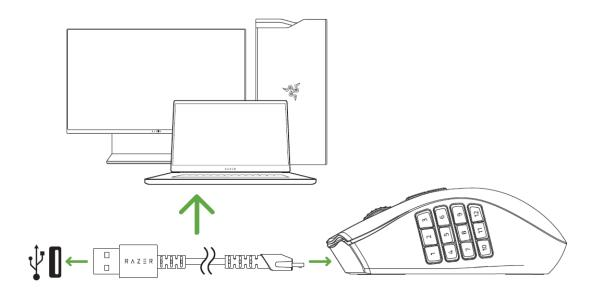
The Razer Naga Pro requires a USB connection that can supply sufficient power to charge the device. The charging process may be affected when connecting to a non-powered USB hub or non-powered USB mostly found on keyboards and peripherals. It's recommended to always connect the Razer Naga Pro directly to the USB port of your computer.
