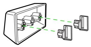
To install the Razer PBT keycap into the stabilizer bar, insert one end of the bar into the stabilizer and use a flat head screwdriver to nudge and hook the other end into the stabilizer.
