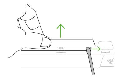
• You may temporarily remove surrounding keycaps to make the removal and/or installation of keycaps and/or stabilizers easier.
