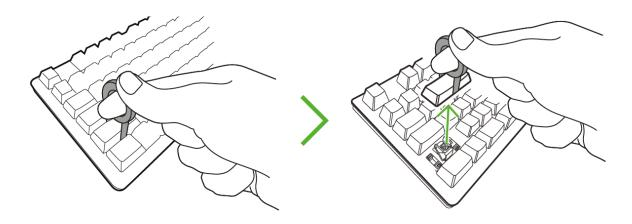
2. (For larger keys) On its corresponding Razer PBT keycap, insert the required optical keyboard stabilizers into its stems.
