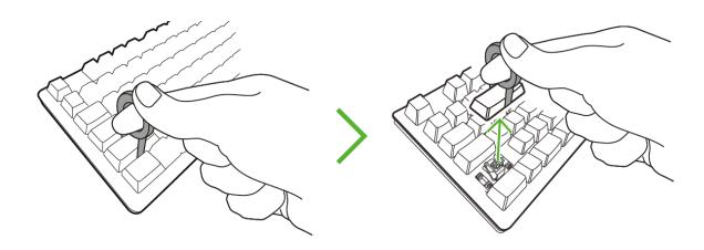
(For larger keys) Gently lift the detached keycap and nudge any of the curved ends of the attached stabilizer bar outwards using a flat head screwdriver (not included) to release the keycap.
