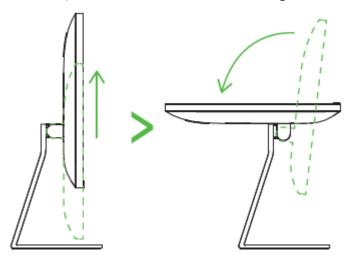
Caution: The monitor has an auto raise mechanism that prevents the screen from tilting at extreme angles. Do not force the screen to tilt 90-degrees when it is at the lowest point, doing so may cause serious damage to the external parts of the monitor; and void its warranty. Do not put your hand near the hinge cover or railings to avoid injury.
