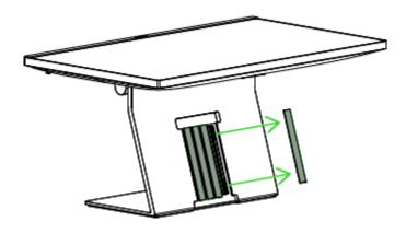
3. Insert the cables through the hole and then plug them to their respective ports.
