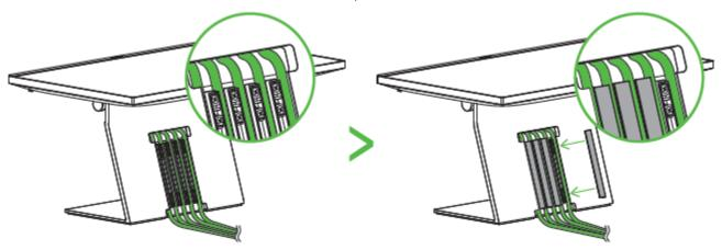
5. Tilt the screen upright while bending the cables inwards for a cleaner aesthetic.
