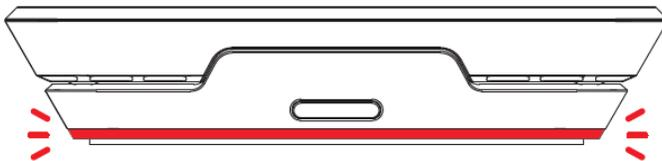
**!** If the underglow lighting continuously flashes in red due to a charging error, check if your device is compatible and/or properly placed at the center of the charging surface.
