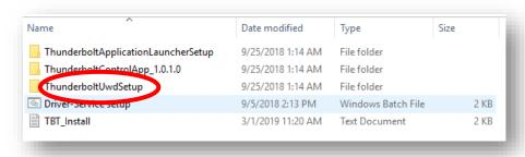
2. Upon clicking on the Driver-Service setup.bat (Windows Batch File), you will be met with confirmation of system changes by the User Account Control window. Click 'Yes' to confirm. Once done, a Windows Terminal Shell window will appear and install the Thunderbolt driver software. The Windows Terminal Shell window will present you with a "Press any key to continue...' message. Press any key as instructed to complete the install.
