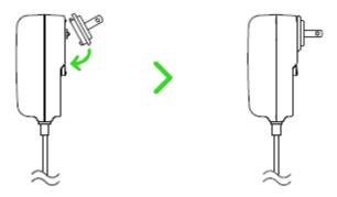
2. Plug the power adapter from your speakers to an appropriate power source.
