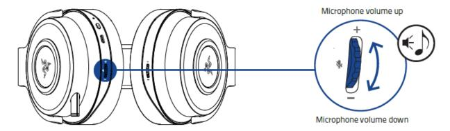
Press the mic volume control to mute or unmute the microphone. The microphone LED will light up when muted.
