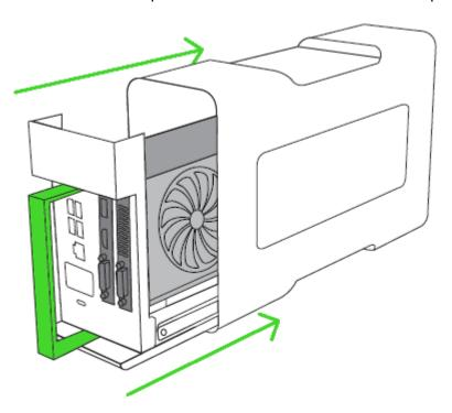
9. Push the lever to lock the compartment.
