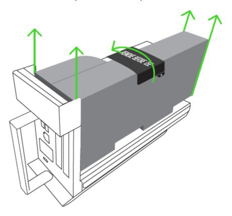
4. Remove the PCI-E slot cover and thumbscrew.
