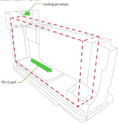
\*Height is measured from the bottom of the locking pin ramps to the top of the PCI-E port.
