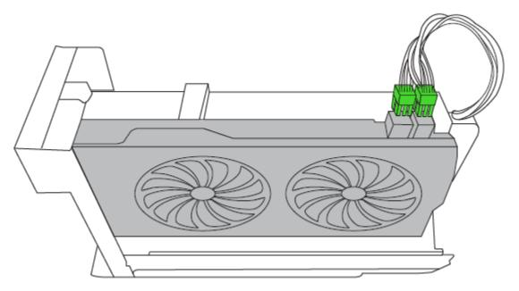
8. Push the compartment into the enclosure until completely shut.
