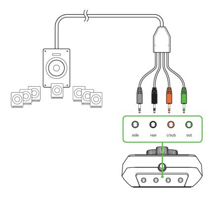
This allows you to use the headset / speakers toggle button to quickly switch between the Razer Tiamat 7.1 V2 and an external surround sound speaker system.
