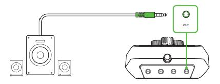
This allows you to use the headset / speakers toggle button to quickly switch between the Razer Tiamat 7.1 V2 and an external stereo speaker system as shown in Fig. 8.
