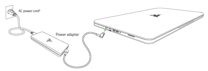
Make sure that the AC plug is properly inserted into the power outlet and the power adapter. An indicator will light up to show that the adapter is receiving appropriate power. Insert the power adapter's connector into the Razer Blade Pro's power port. Press the power button to turn on your Razer Blade Pro.
