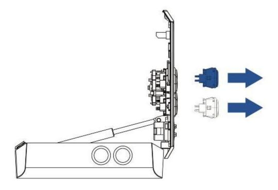
6. Insert your desired action buttons or button covers\* into the slots.
