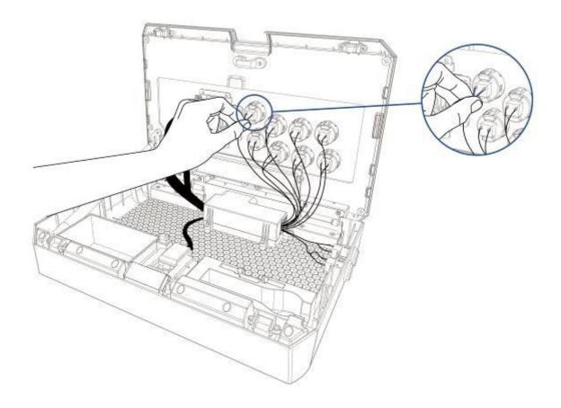
8. Ensure that all cables are properly connected then close the lid.
