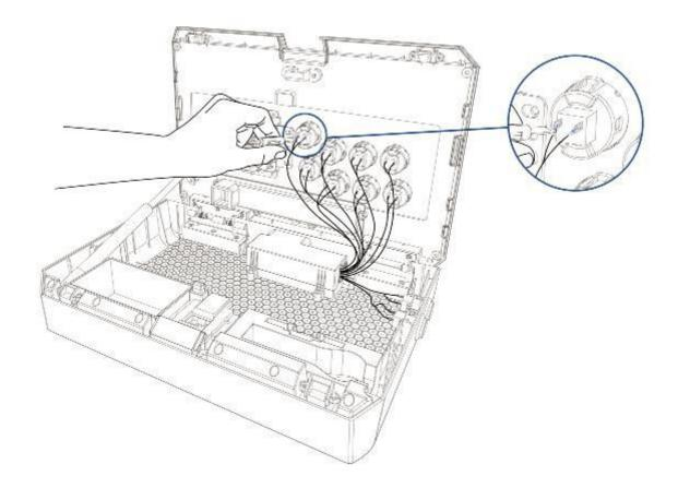
4. While holding the action button's fastener, push the action button out. You can use the screwdriver to push the fasteners in more easily, if needed.
