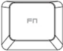
Pressing the “FN” key in combination with the function keys will activate their secondary features.
