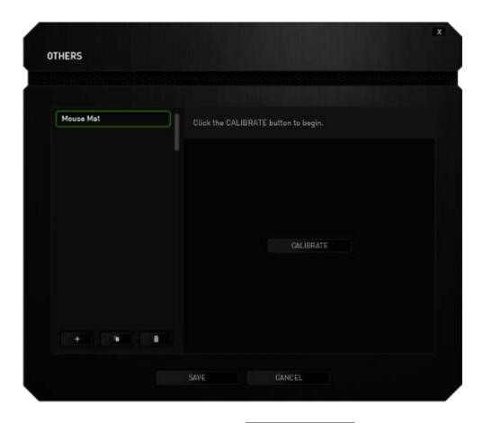
To begin calibrating the sensor, click the **CALIBRATE** button. After clicking the button, Razer Synapse will begin tuning the sensor. Please avoid moving the Razer Diamondback during this time.
