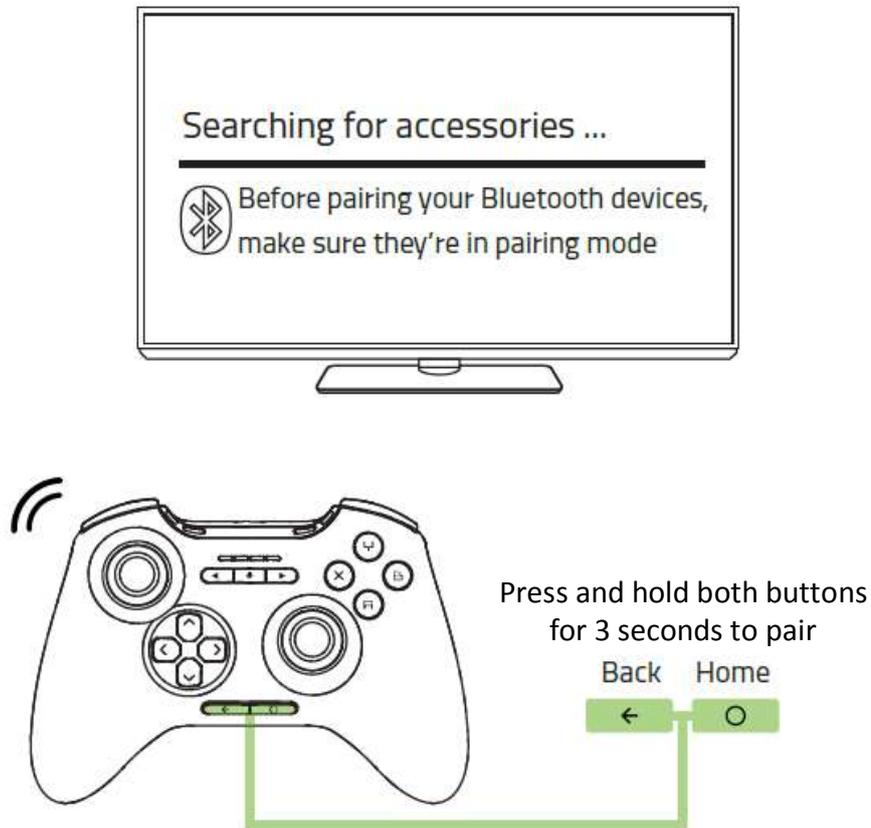
All 4 LEDs will blink simultaneously to indicate that the controller is attempting to connect with the Razer Forge TV. Once paired, you only need to press the **Power** button for half a second to turn on the controller.
