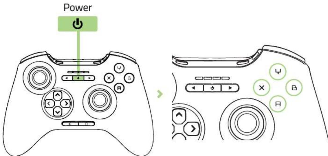
A corresponding LED will blink 3 times to indicate that the device is successfully saved.
