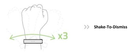
You can manually stop an alarm by doing a Shake-To-Dismiss gesture.
