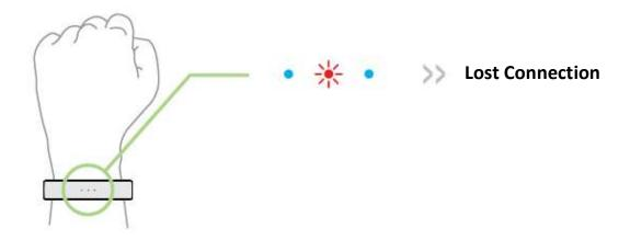
To re-establish a connection, simply open the Nabu X Utility App and bring the Nabu X closer to the paired device.
