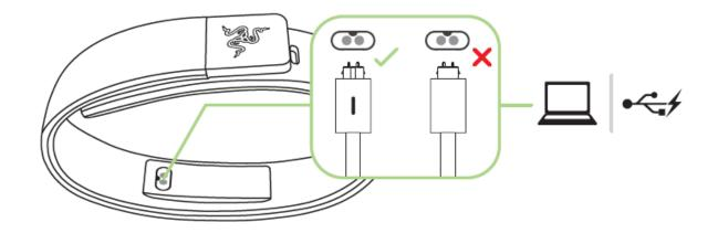
Note: To turn ON your Nabu X you will need to plug it to a power source using the charging cable provided. Do not leave the Nabu X charging overnight. The approximate time to fully charge the Nabu X is 2 hours.
