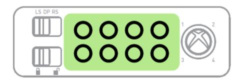
**Turbo 1**: To activate Turbo 1, press the turbo button once. The turbo button will have a steady light to indicate that turbo 1 is activated. When held down, the corresponding action button will perform an action four times (4x) every second.
