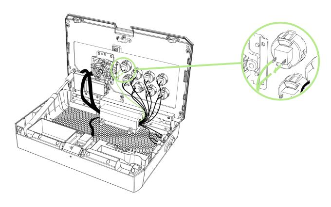
7. While holding the action button's fastener, push the action button out.
