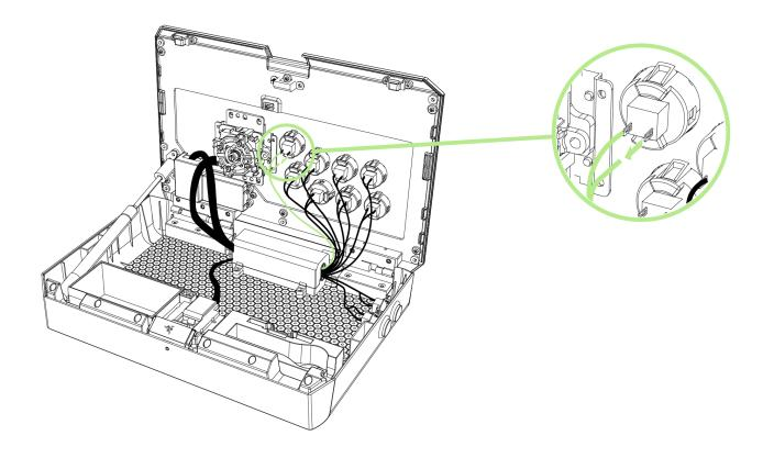
20. Ensure that all the cables are properly connected then close the lid.
