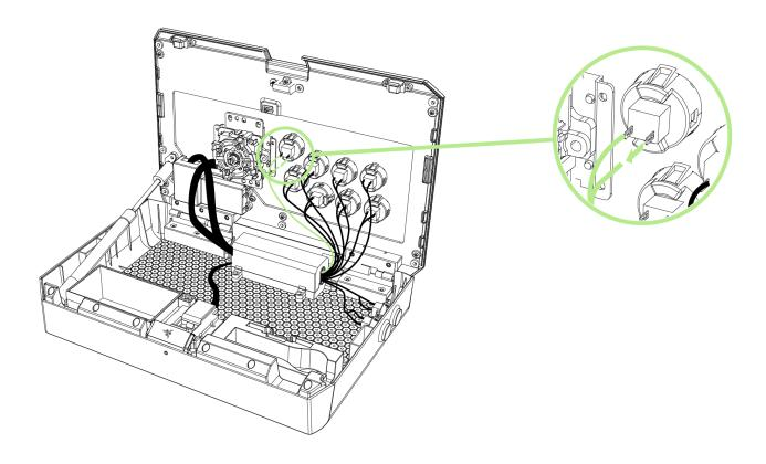
4. While holding the action button's fastener, push the action button out.
