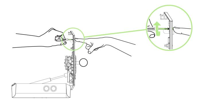
10. Repeat step 9 until all screws and metal stoppers are removed.
