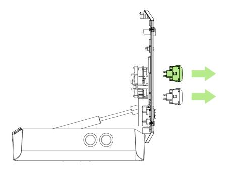
6. Insert your desired action buttons or the button covers\* into the slots.
