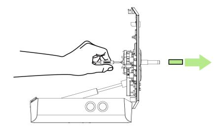
6. Rotate the Bat Top Grip onto the joystick shaft until it is securely fastened.
