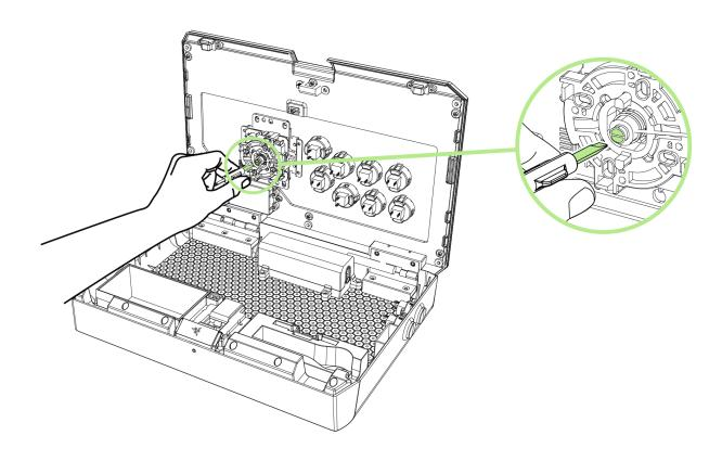
4. Rotate the Ball Top Grip until it is removed from the joystick shaft.
