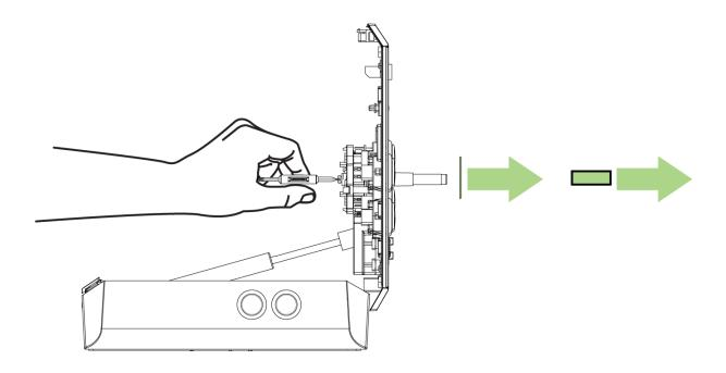
6. Carefully remove the cables from the action button.
