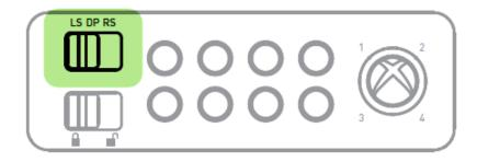
**Note:** To navigate the Xbox 360 Dashboard, set the Control Stick Switch to Directional Pad (DP).
