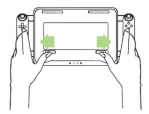
2. Remove the battery compartment door.
