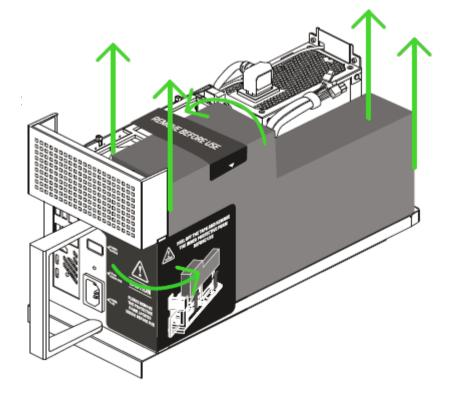
Peel off the stickers and remove the protective foam.
