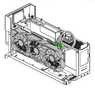
Slide the compartment back into the enclosure then push the lever to lock.
