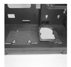
You can also mount a drive on the side exterior of the chassis.
