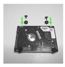
You can mount up to two 2.5" drives on the bottom interior of the chassis.
