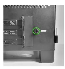
Slide the screw to the right to open the panel and then tighten the screw to keep it secure.
