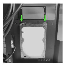
Then, attach the included thumb screw beside the drive to keep it in place.
