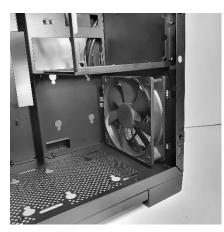
The back can accommodate up to a 120mm radiator and fan.
