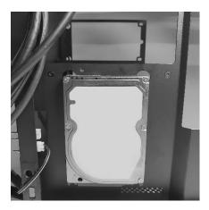
To mount a drive, place the anti-vibration rings between the mounting holes then slide the drive to hold it in place.
