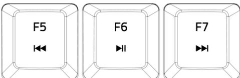
Three keyboard keys: F5 with a double left arrow icon, F6 with a play/pause icon, and F7 with a double right arrow icon. | 您可以使用多媒体键播放/暂停播放 (▶  ) 曲目或向后 (◀◀) 及向前 (▶▶) 跳过曲目。 |
