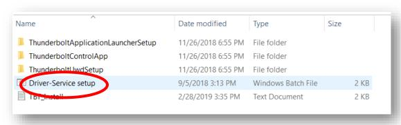
2. Upon clicking the Driver-Service setup.bat (Windows Batch File), a Windows Terminal Shell window will appear with the message that it is installing the Thunderbolt driver. After a few moments, the window will display the message 'Press any key to continue . . . ". Press any key as it instructs, and the install of this driver will be complete.
