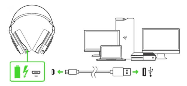
For best results, please fully charge the headset before using it for the first time. A depleted unit will fully charge in about **4 hours**.
