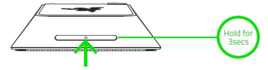
3. From a power off status, press and hold the headset power button for at least 3 seconds.
