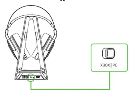
2. Connect the audio hub to your PC using the USB to Micro-USB cable.
