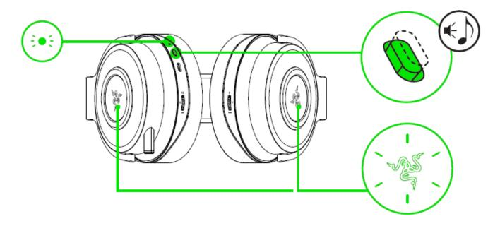
Press the audio hub power button to turn it on. The power indicator will blink until it connects to the headset.
