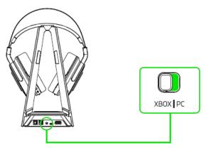
2. Connect the audio hub to your Xbox One using the USB to Micro-USB cable.
