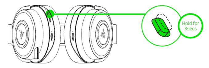
Note: The power indicator on the audio hub, and the Razer logo and the LED indicator on the headset will blink rapidly to show that they are in pairing mode. Keep the pairing devices within close proximity of each other for a faster and more stable connection. If the headset is not paired, it will automatically power off after a few minutes.
