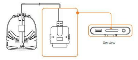
2. Connect the HMD & USB cable to the Belt Box Module.
