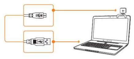
4. Connect the IR camera sync plug to the IR Positional Tracking Camera.
