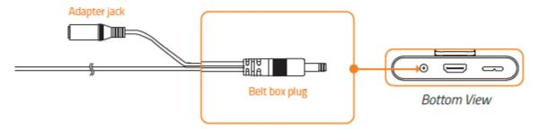
5. Connect the Adapter jack of the Split Cable into the power adapter's Adapter plug and then plug into a power outlet.
