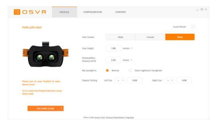
The Profile tab also allows you to quickly configure your interpupillary distance, eyesight, and dioptre settings using the demo scene.
