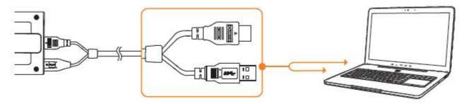
4. Connect the Belt box plug of the Split Cable into the Belt Box Module.
