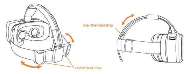
Note: Tightening the over-the-head strap can reduce the pressure of the HMD onto the nose and face. If you feel that you can't breathe properly or that the device is pressing too hard on your cheekbones, the strap is set too long. This will also help redistribute the weight to make the device feel lighter
