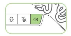
To fine-tune the master volume, press and hold the audio control button then press the directional pad's up or down button to increase or decrease the volume respectively.
