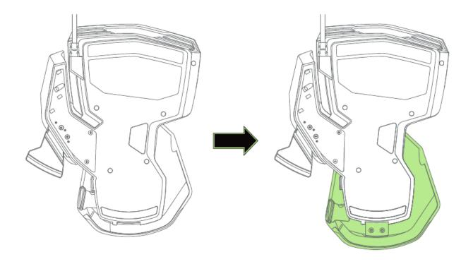
3. Release the lever to lock the wrist rest into position.
