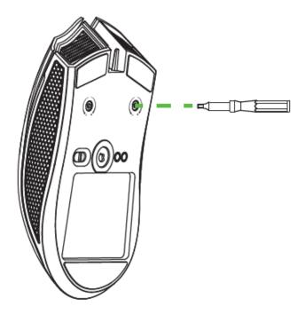
2. Rotate the screwdriver clockwise to increase or counterclockwise to decrease the resistance.
