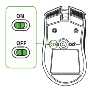
3. To charge the Razer Mamba in wireless mode for best results, ensure that the switch is set to Wireless OFF position and then place the mouse on the charging dock.
