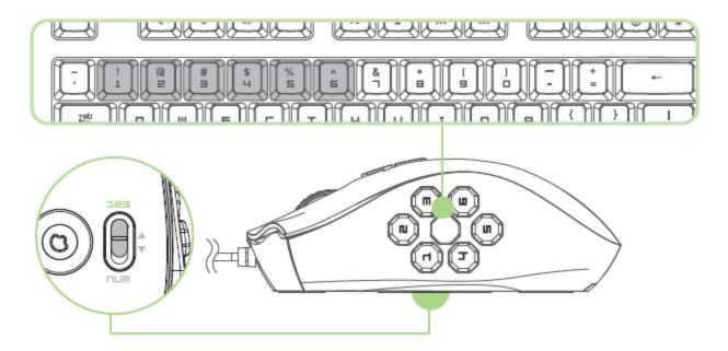
In Basic [123] mode, the 6 Mechanical Thumb Buttons works the same as a keyboard's numerical keys. These buttons allow you to replicate the action bar of most games onto the thumb grid buttons.
