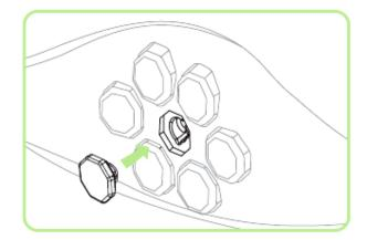
2. Use the indentation to align the thumb rest and the hole.
