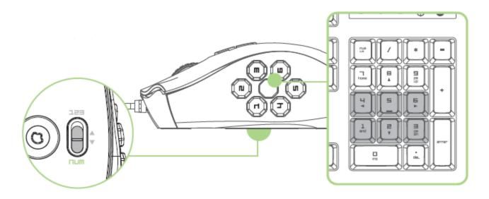
In the Advanced [Num] mode, the 6 Mechanical Thumb Buttons work the same as a keypad's numerical keys. These buttons allow you to have quicker access to in-game commands without having the need to reach for the keypad.
