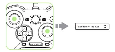
3. Press the up or down arrow to adjust the sensitivity.
